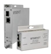
The TMC-GSFP electrical-to-optical Ethernet media converters accept a 10/100 or 1000 Mbps electrical input and converts to a 100 or 1000 Mbps optical output (selected by a dip switch) and the 100/1000 Mbps optical input back to the 10/100/1000 Mbps electrical output. "Auto-Negotiating" is supported on the copper interface side. These devices use either one or two optical fibers, depending upon the selection of sold-separately SFP<sup>†</sup> optical module.
